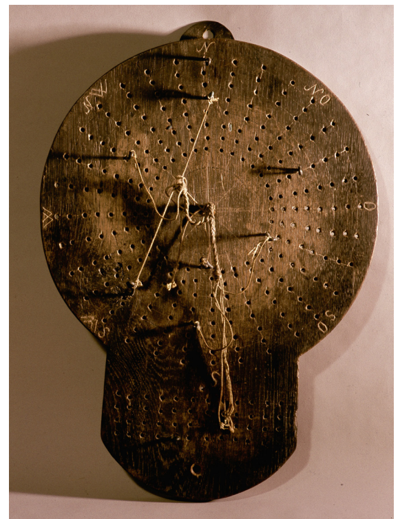
A traverse board that was used to keep track of a ship's speed and direction for four hours at a time. The large circle is the compass rose, and below it are four rows, each representing a half hour of travel. © Getty Images.
